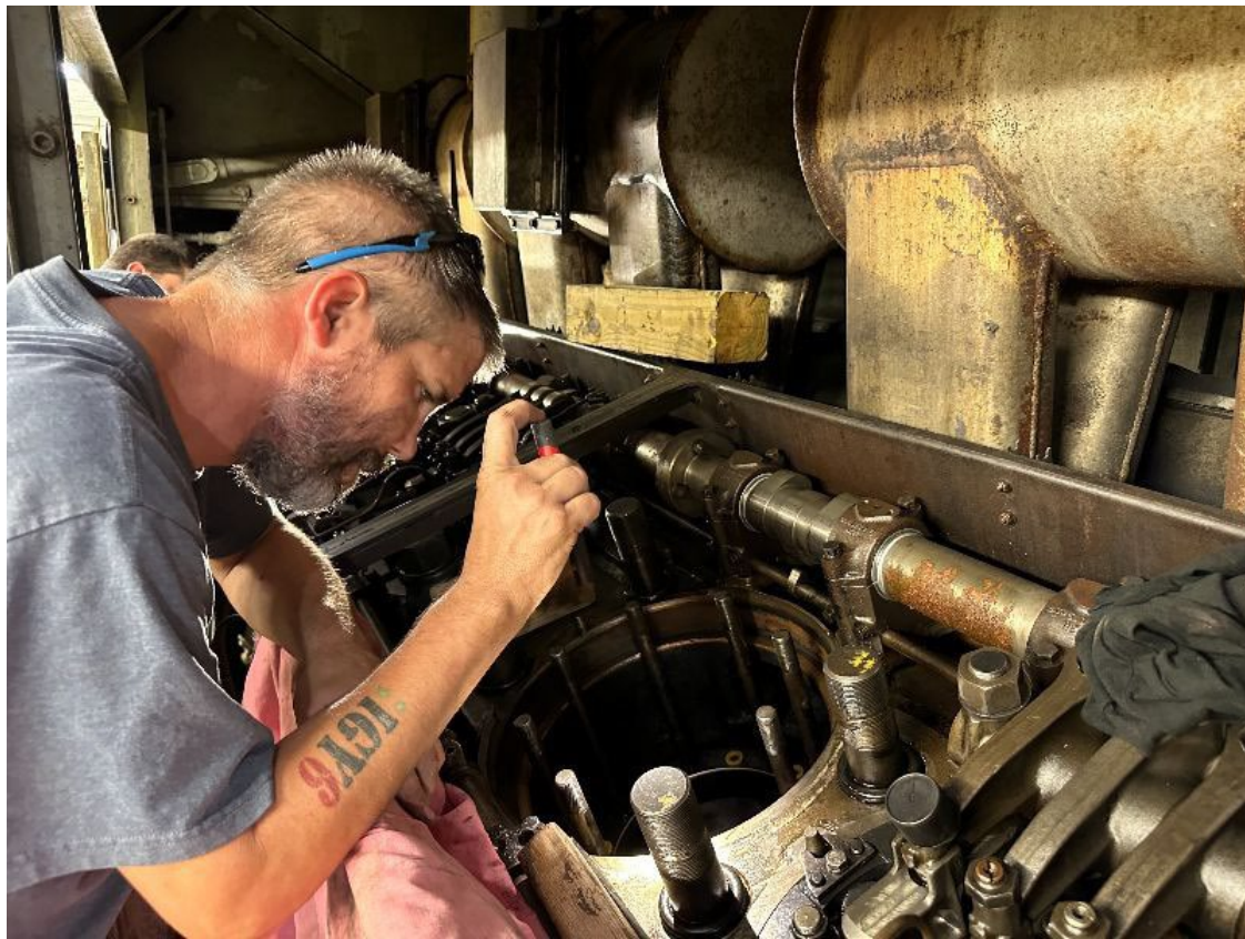
Volunteer John Nave works on cleaning a cylinder liner for reinstallation on the head on our CF7 locomotive.
