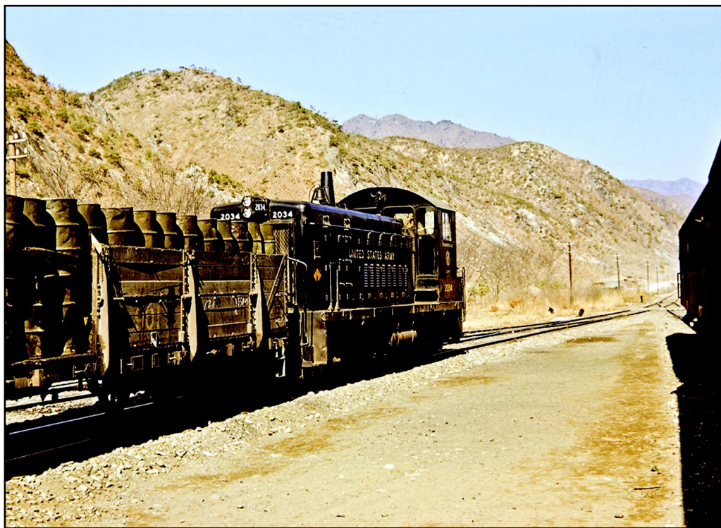
EMD SW8 Diesel Locomotive powered supply train operated by the 712th TROB taking supplies to the front lines during the Battle of White Horse Mountain. Note locomotive number 2034 matches that on the first insignia depicted (Courtesy of Mr. Dewey MacLean)
